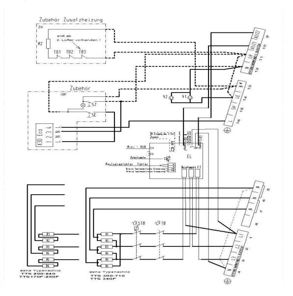
Important! Do NOT connect Terminal 13 to power supply if an integral thermostat Type IRT 24Z is being use
